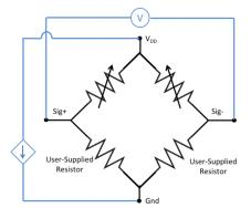
In this configuration, a constant voltage is maintained between Vdd and Gnd and the voltage drop from Sig+ to Sig- is proportional to pressure.
